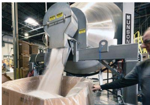
Internal flights direct blended material toward and through a plug-gate valve with no stratification into a Gaylord on a scale. Source: Munson Machinery
